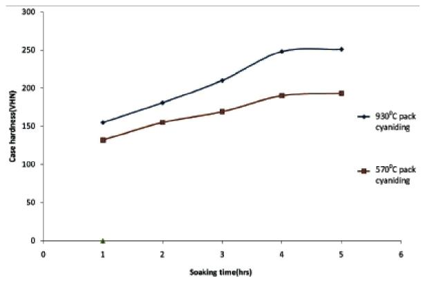
Fig. 4: Case Hardness with respect to soaking time for 570°C and 930°C Pack cyaniding
